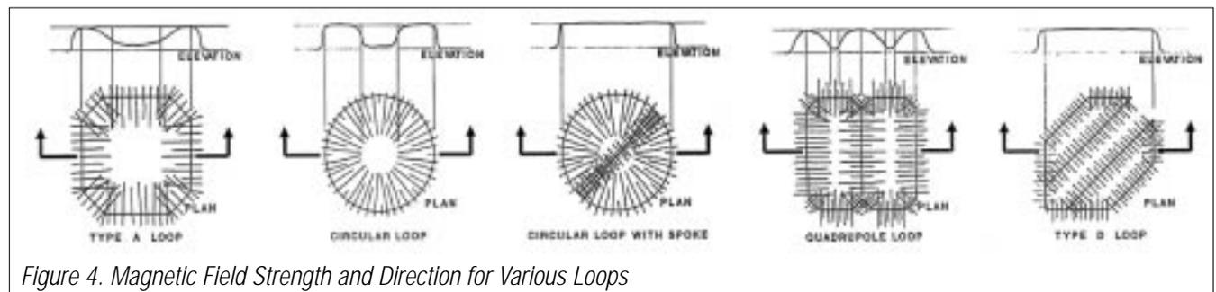
Figure 4. Magnetic Field Strength and Direction for Various Loops
