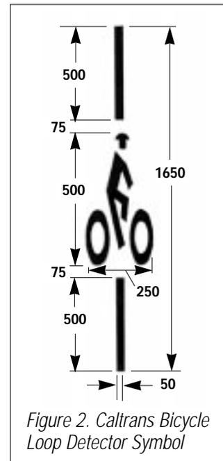
Figure 2. Caltrans Bicycle Loop Detector Symbol
