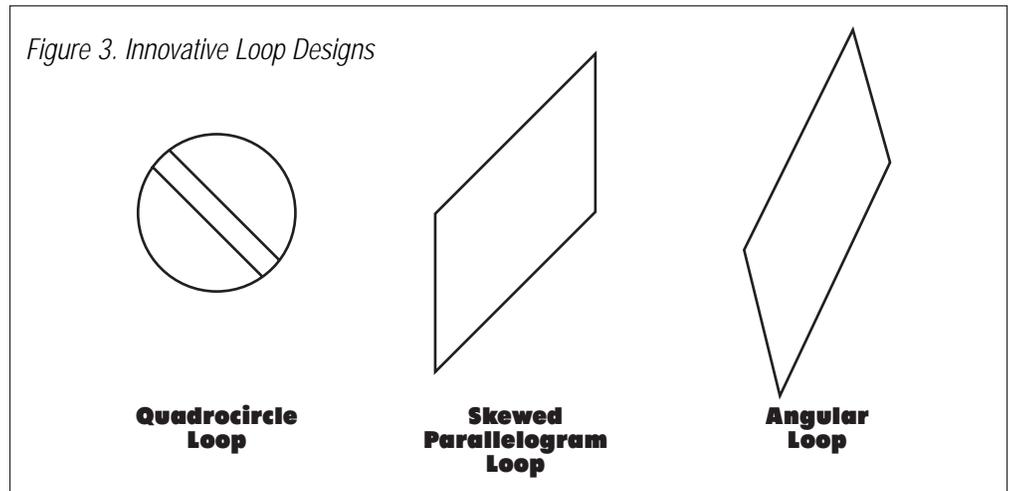
the loop shape. This concentration increases field strength for same-lane detection and minimizes spillover, enabling the use of higher detector sensitivities.
